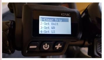
To reset the trip and access some advanced settings, press and hold both button either side of the power button for a couple of seconds.
