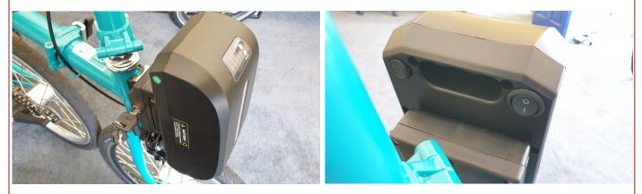
The battery has a meter showing the remaining capacity, and a light which would normally be used when the battery is fitted to the rear of a bike. To see the state of the battery, press the 'Voltage' button, and to switch the light on/off, press the light button. The light will cycle from Off > On > Flashing > Off.
