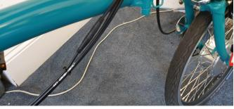
Shrink the supplied heat-shrink sleeving over the battery cable connectors, and then use the ribbed cable-tidy to secure/hide the cables.
