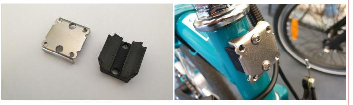
The parts to be fitted next are shown below-left. Drop the white into the rear of the black casing, and feed the four M5 cross-head bolts through the metal support from the other side, and then secure it to the bike. The round opening in the side of the black plastic should be on the left as you look at the bike (the right side if you were sitting on the bike).
